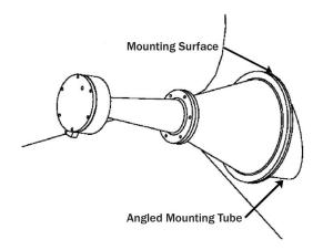
B. <u>Mounting surface sandwiched between bell sections</u> – The horn is mounted such that the end of the last or middle bell section protrudes inside the vessel.
